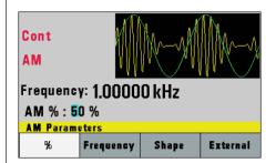
The 4045B provides AM and FM modulation along with linear/logarithmic sweep and built-in counter capabilities. Internal and external sources can be used for triggering and modulating the signal.
